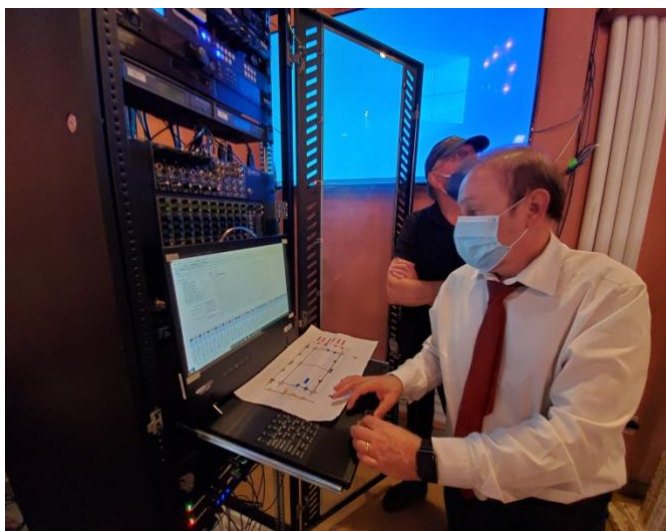
LIGHT CHECK... CEO Ganim Hanna works from laptop to make studio lighting adjustments during the trial. Each light can be individually illuminated, dimmed or brightened through this control box. Production Specialist Leonard Cummings (background) watches each studio instrument's response to inputs from Ganim.
